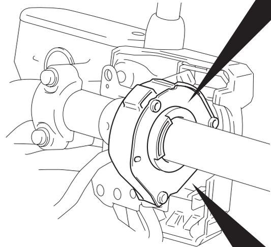
Be careful not to adhere grease to the outside of dimensions shown.
