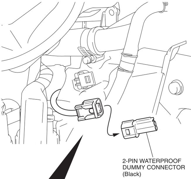
Remove the connector from the clip as shown.
