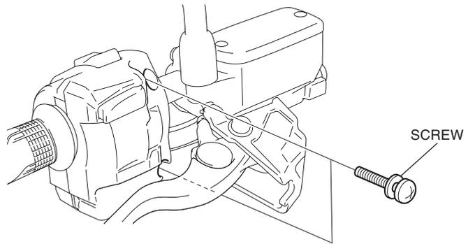
35. Remove the right front housing as shown and remove the screw.
