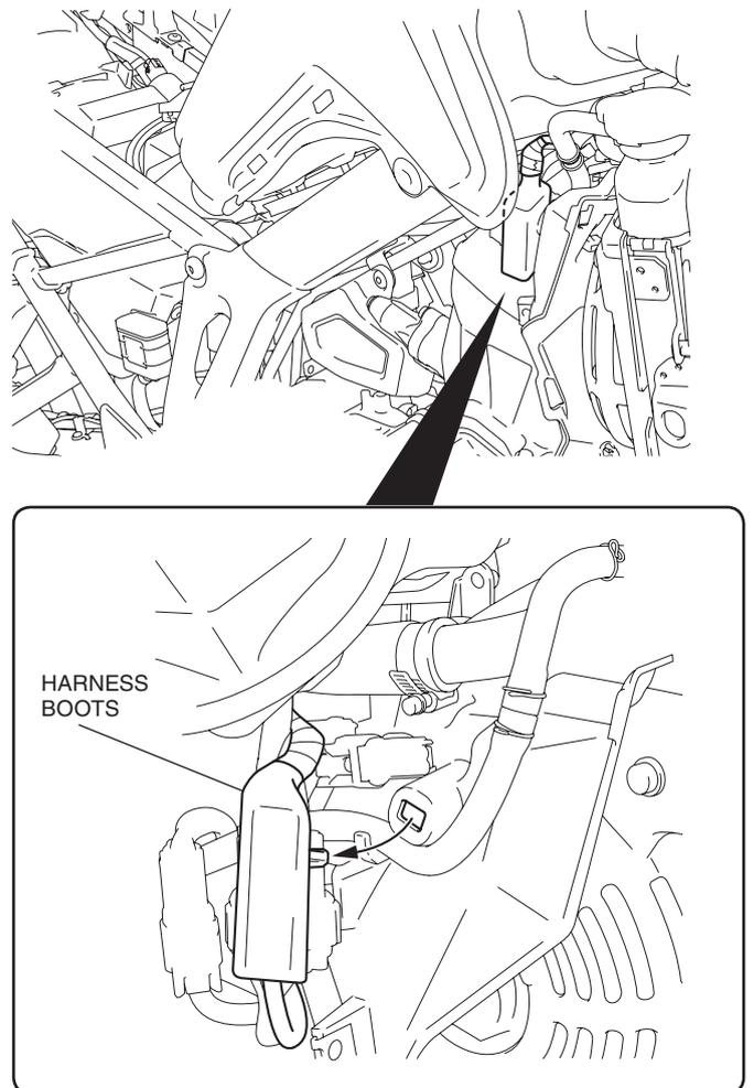
50. Remove the dummy connector as shown.
