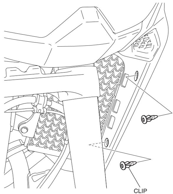
6. Remove the front tank cover as shown.
