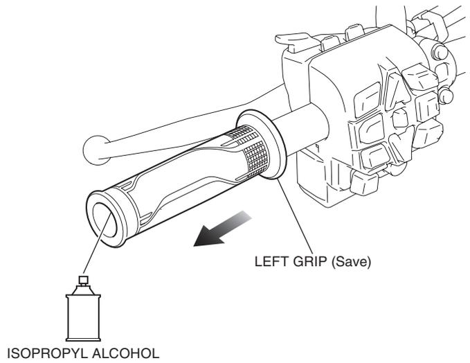
19. Using an isopropyl alcohol, remove all traces of adhesive from the left handlebar.
