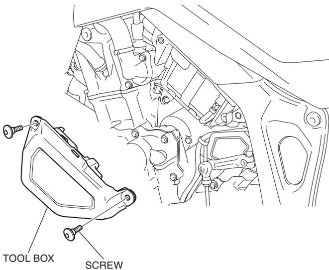
4. Remove the screw as shown.
