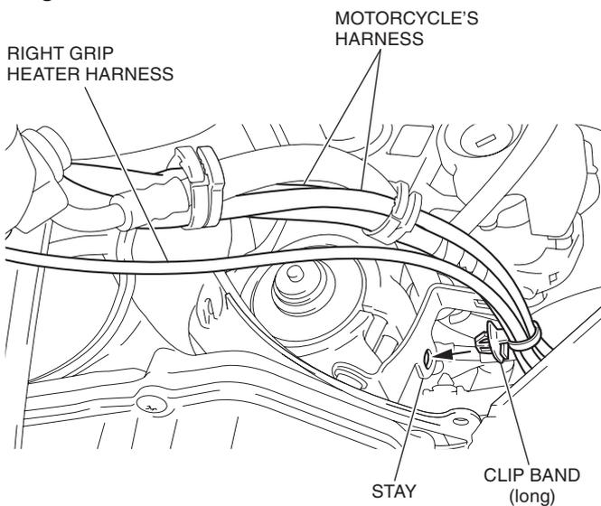
70. Secure the right grip heater harness with the clamps as shown.
