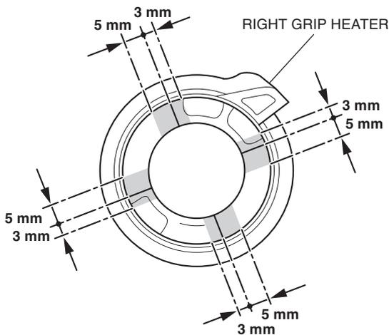
39. Apply grease to the hatched part as shown.
