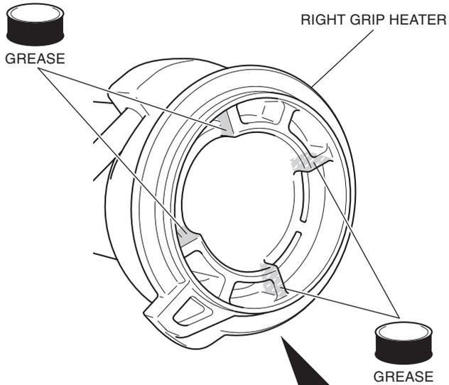
Be careful not to adhere grease to the outside of dimensions shown.
