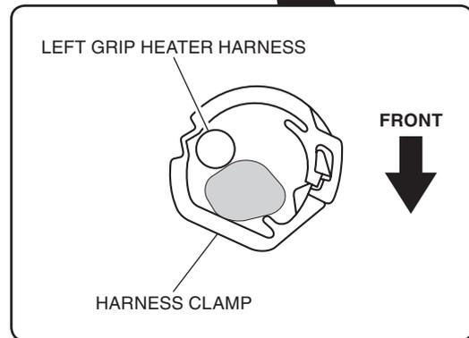
32. Secure the left grip heater harness with the clamps as shown.
