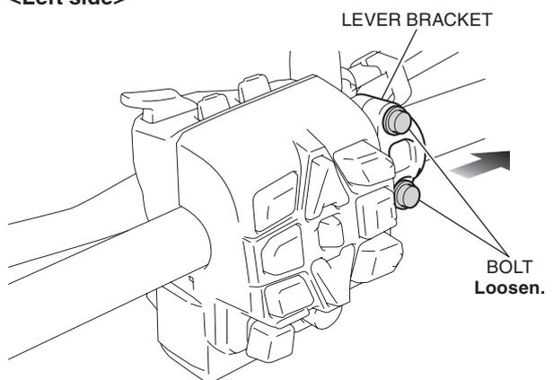
21. Remove the winker switch rear housing as shown.
