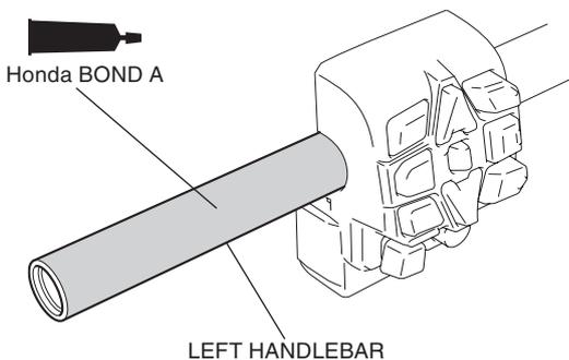
24. Spray isopropyl alcohol over the inside of the grip heater and outside of the left handlebar.
