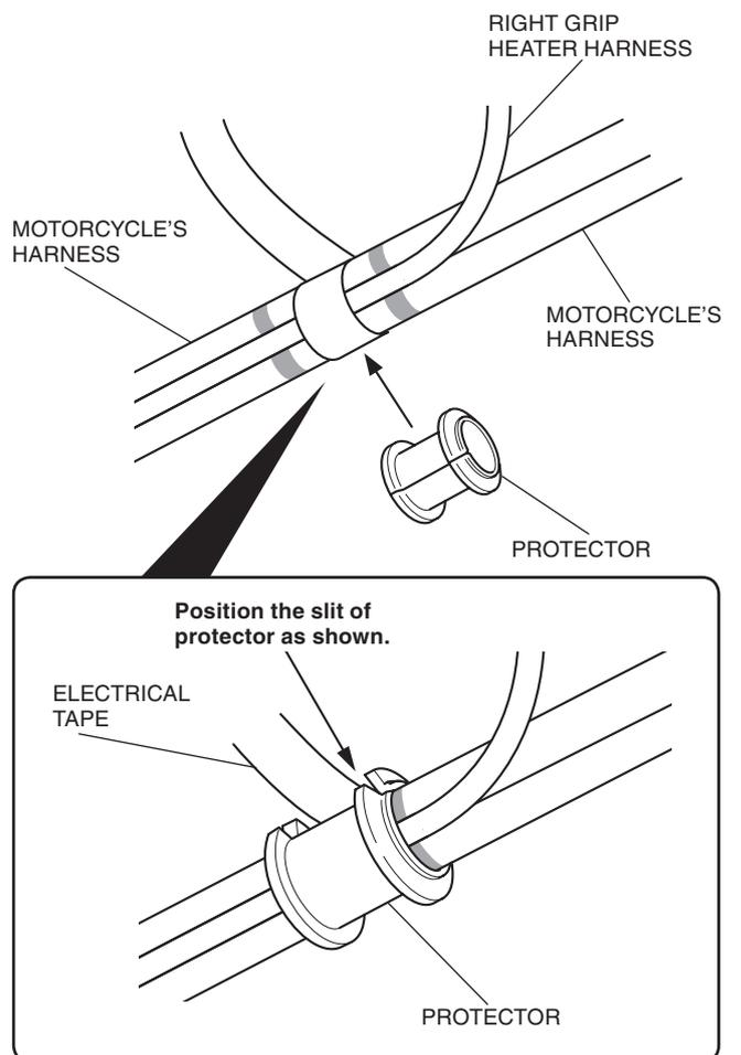
63. Secure the protector with electrical tape as shown.
