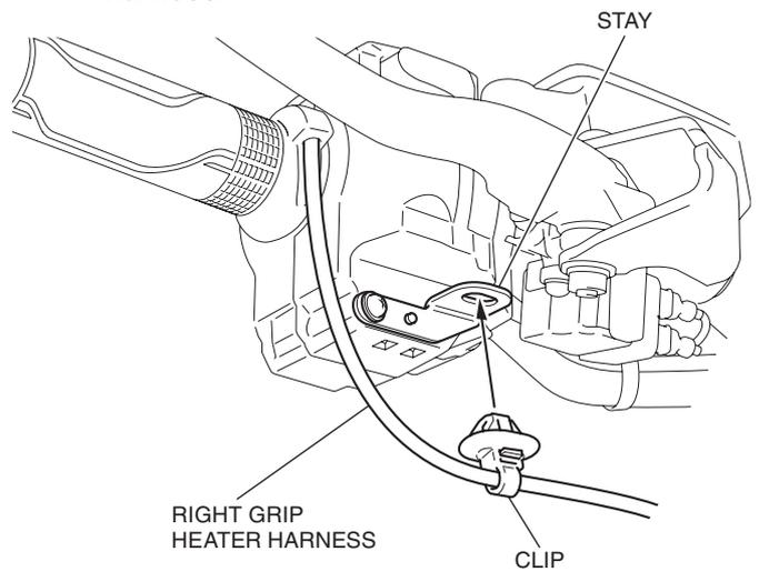
46. Secure the right grip heater harness with the wire tie as shown.
