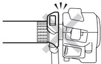
• If the grip gets stuck halfway during installation, apply isopropyl alcohol to the gap between the grip heater. Do not try to remove the grip heater using force or a screwdriver, etc. Damage to the grip heater wire can result.
