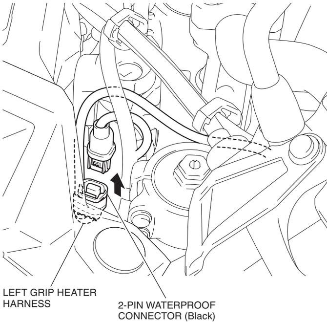
31. Secure the left grip heater harness with the harness clamp as shown.
