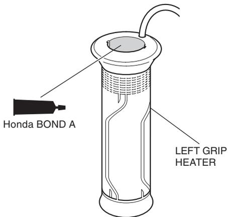
23. Apply the Honda bond A to the left handlebar as shown.
