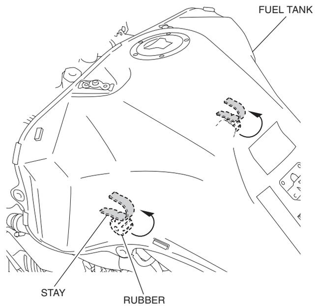
15. Loosely install the fuel tank as shown.
