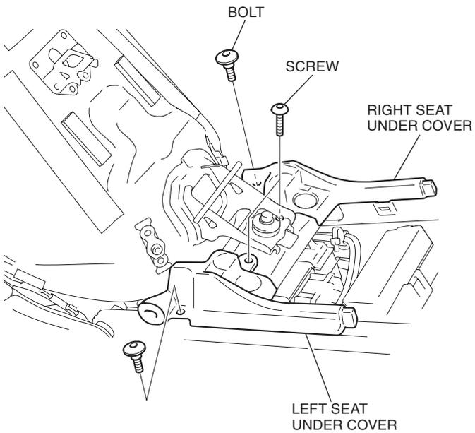
13. Remove the parts as shown.
