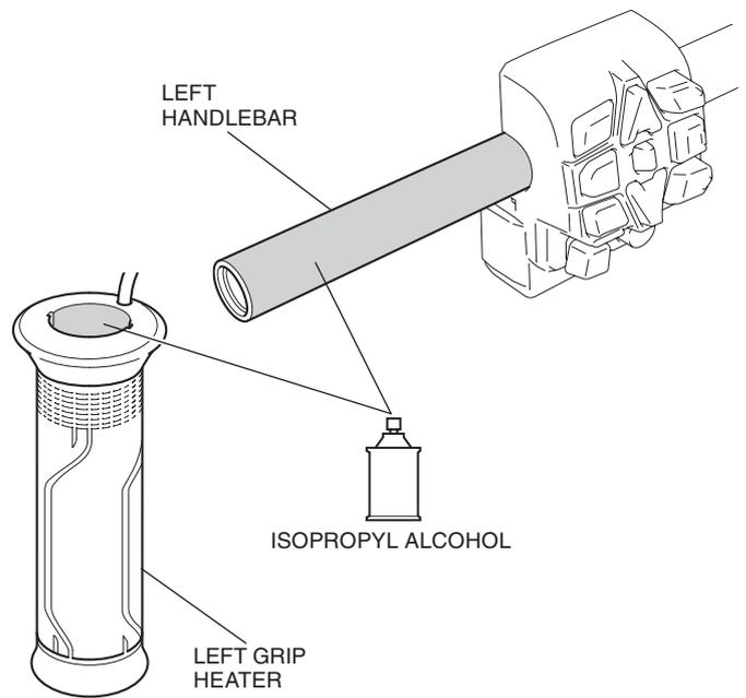
25. Slide the left grip heater onto the left handlebar and route the left grip heater harness as shown.
