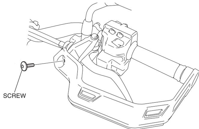
17. Remove the parts as shown.
