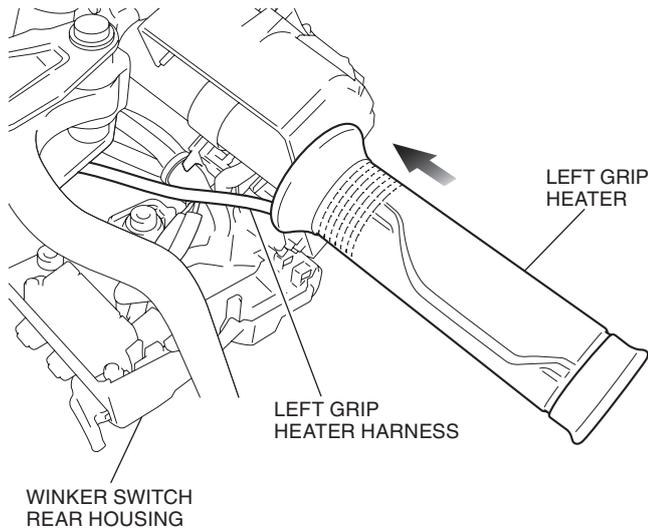
26. Insert until there is contact with the winker switch front housing, then align the indicated position.
